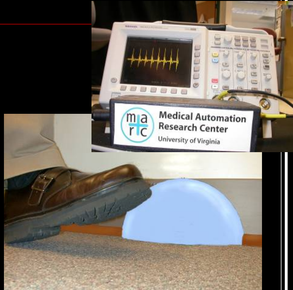
The sensor system shown mounted on the baseboard in walkway path
